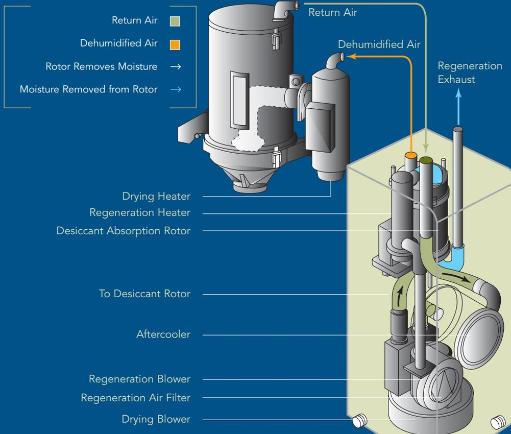
Matsui's desiccant rotor technology has become the industry standard in dehumidifying hot-air drying equipment. Its unique, honeycomb design—molecular sieve desiccant, bonded and then baked onto ceramic paper—eliminates powder that can contaminate the system. Its large contact area effectively absorbs at high temperatures, drying resin in half the time while stabilizing dew points at a constant  $-40^{\circ}\text{F}$ .
