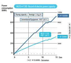
**Resin savings** – Once material in the hopper is warm and dry, the MJ5-I powers down, preventing potential degradation or loss of properties.
