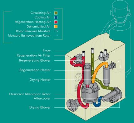
Matsui's desiccant rotor technology has become the industry standard in dehumidifying hot air drying equipment. Its unique, honeycomb design—molecular sieve desiccant, bonded and then baked onto ceramic paper—eliminates powder that can contaminate the system. Its large contact area effectively absorbs at high temperatures, drying resin in half the time while stabilizing dew points at a constant -40°F.
